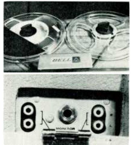
Top: rubber reel locks are provided so that the reels will stay on when the deck is used in the vertical position. Lower: inputs and monitor jacks are on rear of deck. The transport may be used either horizontally or vertically.
