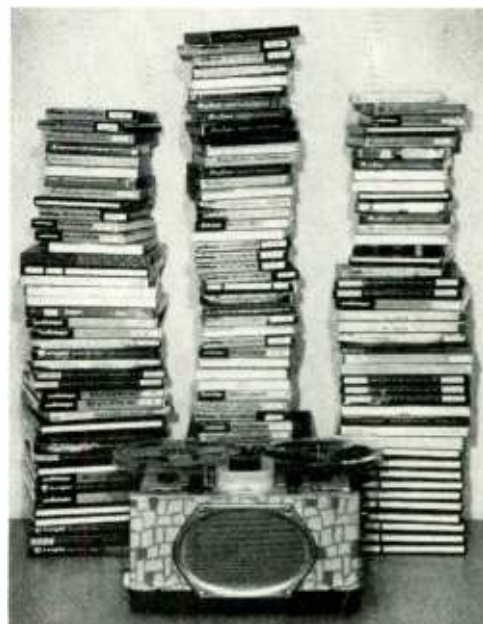
Fig. 2: Imagine the money saved by using three-fourths of this tape over again. Here is a precious personal collection of monaural, twin-track tapes recorded at 7\frac{1}{2} ips. A new recorder can re-record these onto four tracks at 3\frac{3}{4} ips with very little loss in quality, "condensing" everything down to a mere one-fourth in space.
