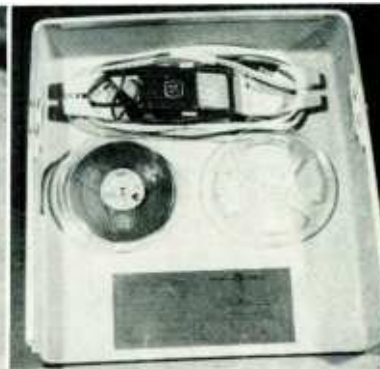
The lid has storage space for the microphone and its cord, the cord for connecting to the power supply and pins which will hold two five inch reels in place.
