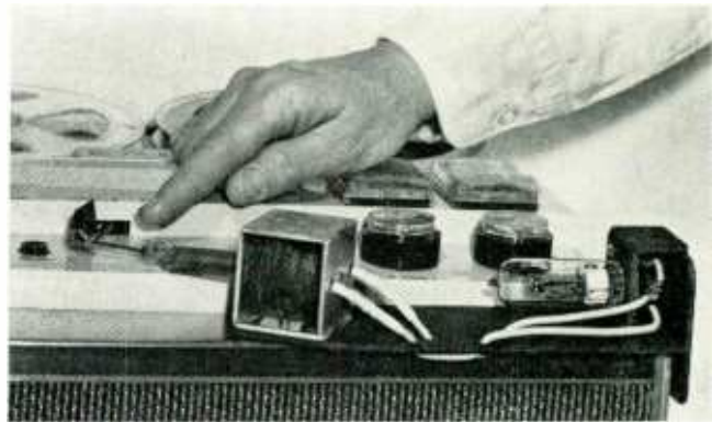
Fig. 10: Another use for a delay relay is in shutting off a "disengager" solenoid immediately after it has done its job, eliminating the need for a timer clock for this function (as described last month). The complete unit, which also includes a tape shut-off switch, is quickly put into use and is just as quickly removable.
