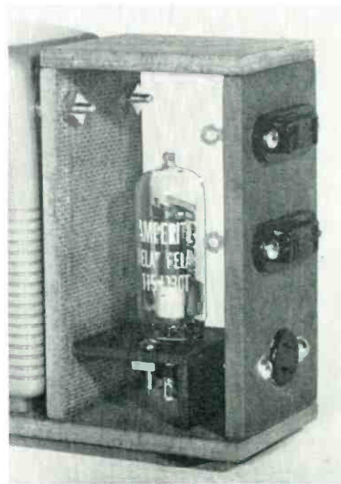
Fig. 5: Although the exact shape and size of the little housing is not too important, be sure to leave adequate room around the relay tube to allow for proper ventilation. The upper two receptacles are regular solder-lug AC chassis sockets, while the lower one is purposely different as it connects directly to the recorder motor.
