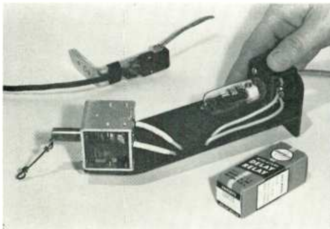
Fig. 11, left: Exactly how you construct the solenoid shut-off device will depend on the recorder you have. All you need, actually, is a support that will hold the solenoid in correct position for working the "Off" lever or knob to disengage the idler wheel, as well as necessary support for the delay relay tube and the needed wiring. Fig. 12, right: When the tape runs out, the tape switch immediately actuates both the solenoid and the heater element of the relay. First the solenoid acts to remove the pressure of the idler wheel and then two seconds later the relay turns the solenoid off. In this case, a delay relay that "opens" instead of "closes" is used for the job.
