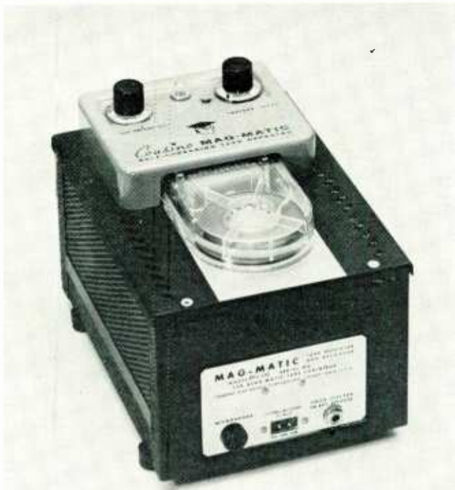
The Cousino machine uses a Cousino cartridge which is a continuous loop of tape. Up to an hour of playing time may be had. A capstan and roller furnish the drive.
